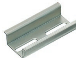
TS 35/15 mm according to EN 50022 (s = 1.5 mm)
