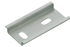
TS 35/7.5 mm according to EN 50022 (s = 1.0 mm)
